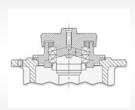
LEXUS Scaife Drive are precision machines for driving diamond polishing Scaife at high speed with high precision, controlling dynamic axial run-out in very tight limits.
