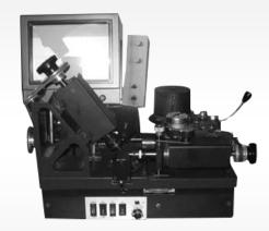
Ultimate Machine for cone bruting from Crown side
