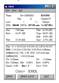
Lexus Dia-analyser, the single camera module, is used predominantly in factories, after pre-bruting, Mainly for parameter distribution and cut class analysis.
